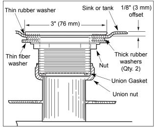
Figure 5. Installing Sink Strainer
